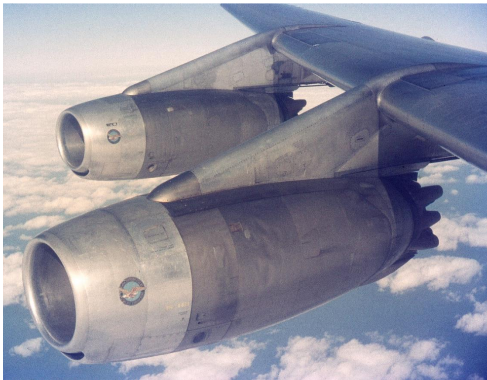
JT4A (installed on DC-8)
