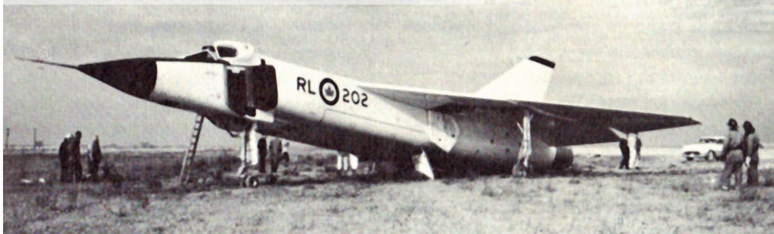
Accident of RL-202 after a landing gear failure (November 11, 1958)
